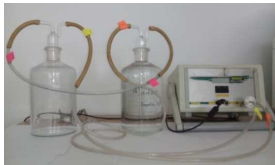
Figure 3. SARAD RTM-1688-2 measuring system for ^{226}\text{Ra} in water
