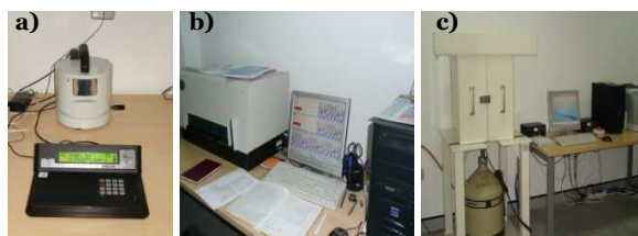
Figure 2. a) Universal device UVJ-01, b) \alpha/\beta counter PIC-MDS-8, c) HPGe – GMX 50P4 detector
