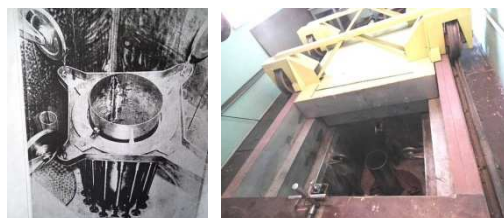
Figure 7. The ^{60}\text{Co} gamma irradiator GOU-1 is operated in batch mode and used mainly for pilot-scale irradiation
