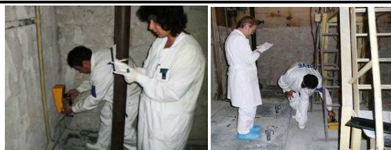
Figure 1. Tracking and record-keeping of RAW - measurements of surface contamination of the primary cooling loop premises
