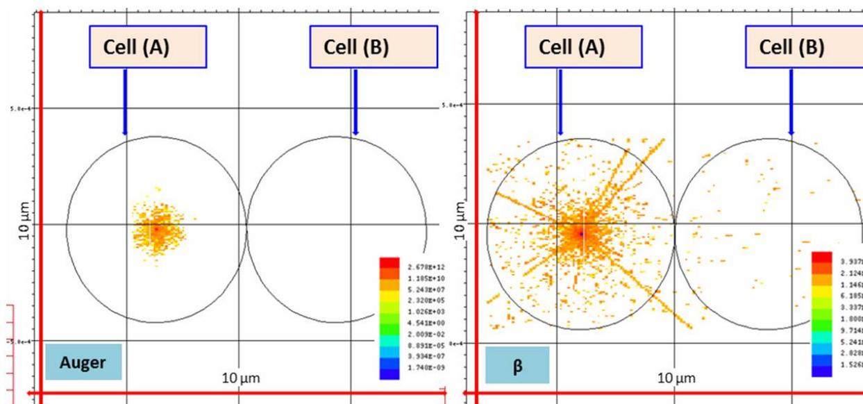
Figure 3. Auger (left) and  $\beta^-$  (right) absorbed dose distributions for  $^{64}\text{Cu}$  radionuclide. The dose values of the Mesh tally are in MeV/g/particle units. The emitting source was placed inside the cell A at 1.10 nm from the DNA axis volume (see section 2.3 for further details).
