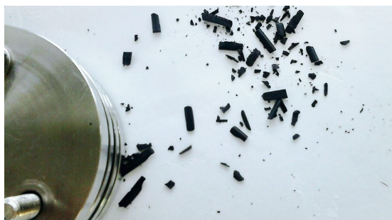
Figure 3. Complete structural failure of EPDM O-ring samples after post-irradiation compression set test. Samples irradiated at about 4 MGy of absorbed dose experience huge radiation-induced brittleness.
