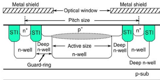
Figure 1. P+/Nwell SPAD structure (see [18])
