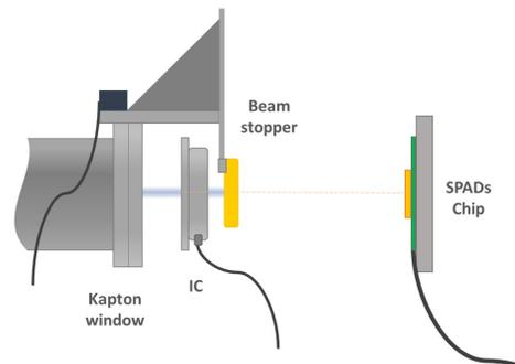
Figure 4. Layout of test beam setup
