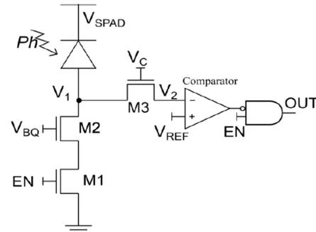
Figure 3. Pixel read-out circuit
