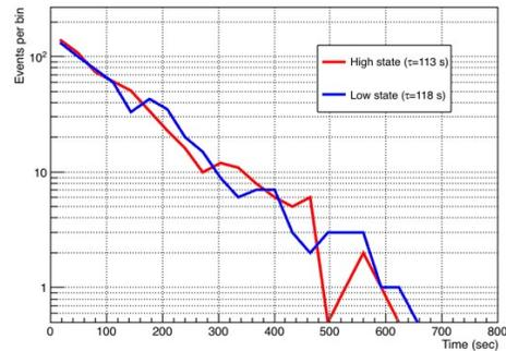
Figure 10. Time spent in a high and low DCR state in a SPAD with a two-level RTS fluctuations
