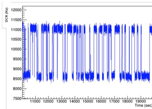
Figure 8. Two-level DCR fluctuations
