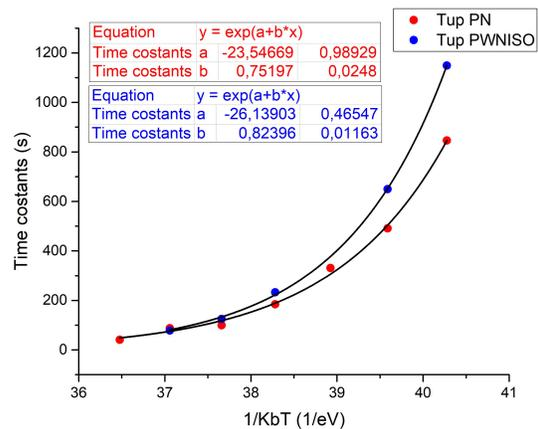
Figure 13. Time constants as a function of 1/KT for high RTS level in two SPAD pixels with a different layout
