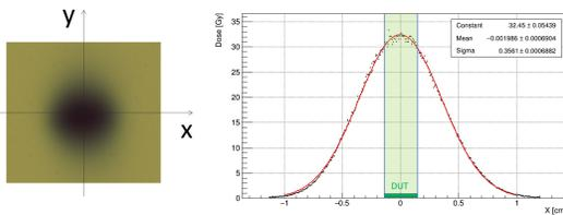
Figure 6. Exposed GAF and proton beam profile
