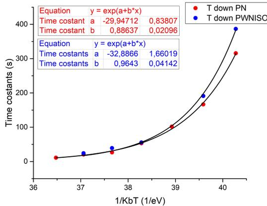
Figure 12. Time constants as a function of 1/KT for low RTS level in two SPAD pixels with a different layout
