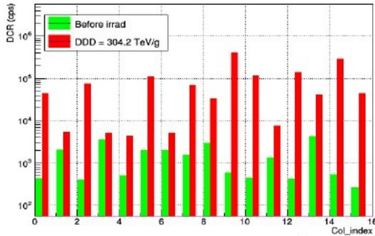
Figure 7. DCR increase after irradiation in 10x10- $\mu$ m SPAD arrays
